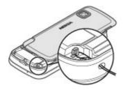
Tip: Attach the plectrum stylus to the device as you would a wrist strap.
